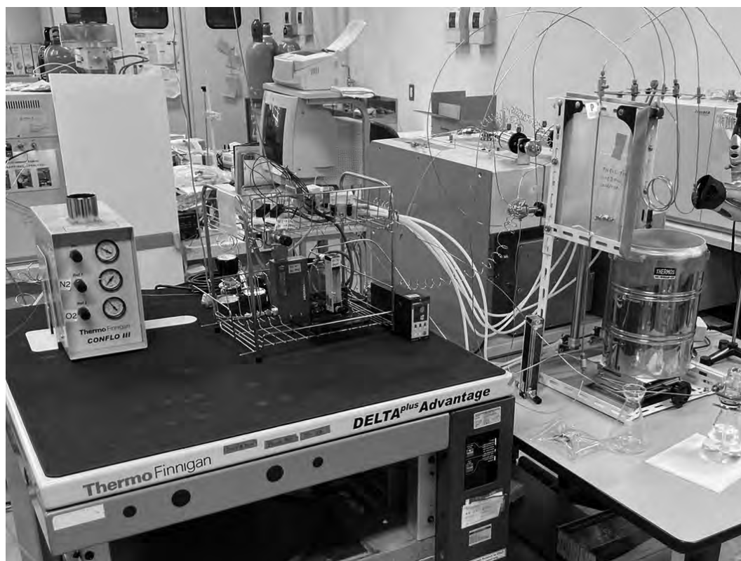
Fig. 2. Measurement system for \Delta^{17}\text{O}(\text{H}_2\text{O}_2) values developed in this study.
