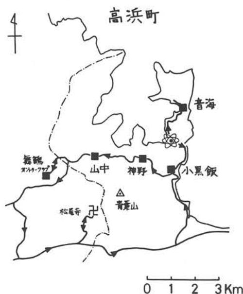
Fig. 1. Route map of carborne measurement in Takahama T. in Fukui prefecture. The black squares show the points of In-Situ Ge(Li) measurement.
