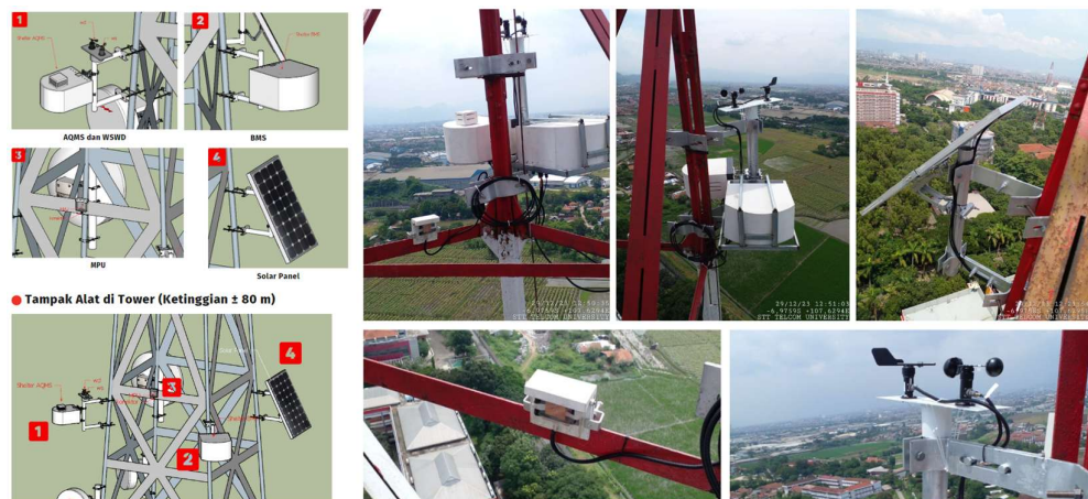
Fig. 5. Design and implementation of telecommunication-tower-based air quality monitoring systems using low-cost sensors.
