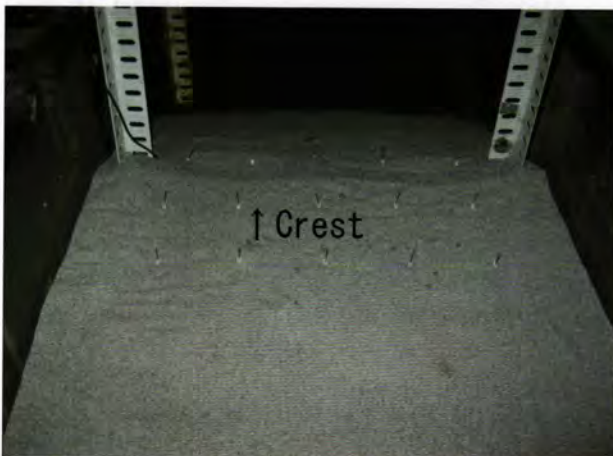
Fig.3 Post-shaking deformation at the crest due to liquefaction.
