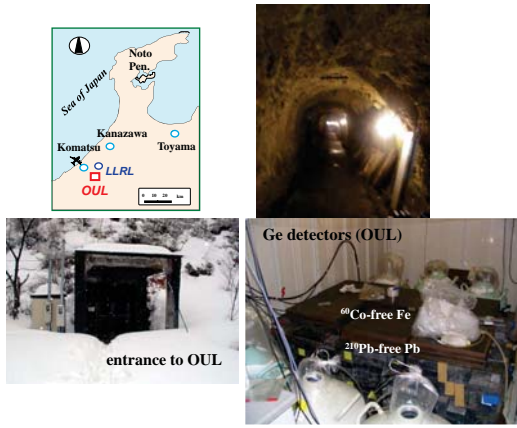
Fig. 1: Low-background \gamma -spectrometry using Ge-detectors in Ogoya Underground Laboratory was conducted in seawater, riverine particle, and sediment samples.
