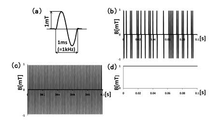
Fig.2 Waveforms of electromagnetic field. (a) A sin wave at 1 kHz with a amplitude of 1 mT was used as a single pulse. (b) Random pulse train (RdPT). (c) Regular pulse train (RgPT). (d) Constant electromagnetic fields (DC).
