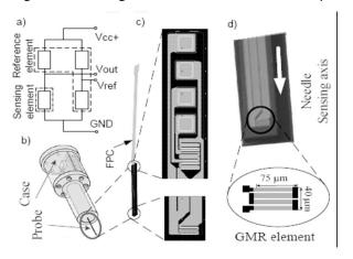
Fig. 4 The SV-GMR probe: a) schema of Wheatstone bridge electrical connections, b) needle type probe with case, c) needle with flexible printed circuit with enlarged needle tip and bonding pad d) microscope picture of needle tip with marked sensing axis of SV-GMR element.
