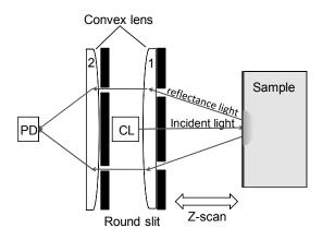
Fig.1 Schematic configuration of bone densitometry using diffuse reflection light. CL: Coherent light. PD: Photo detector.
