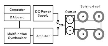
Fig.1 An experimental system for electromagnetic field stimulation to cultured
