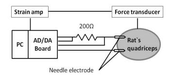
Fig.2 Electric stimulation and muscle contraction force measurement
