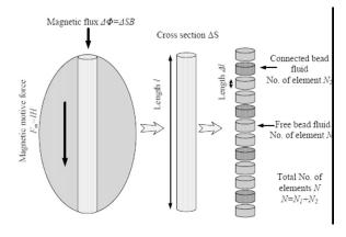
Fig. 2 Magnetic path and permeability of mixed fluids.
