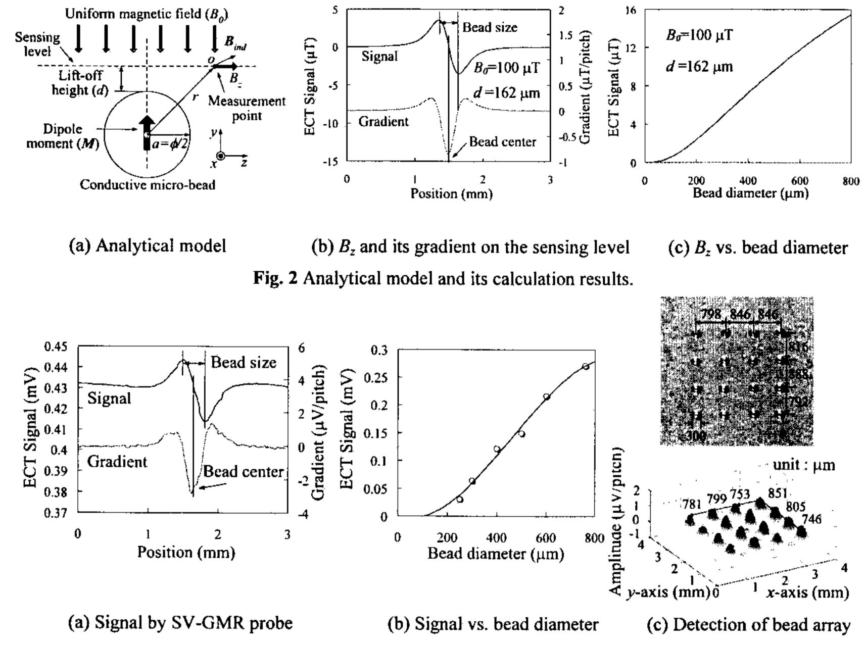
Fig. 3 Inspection signal obtained from SV-GMR sensor and 2D image of bead array.
