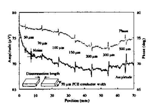
Fig. 4. ECT signal obtained from scanning over 70 µm PCB conductor with conductor disconnection
